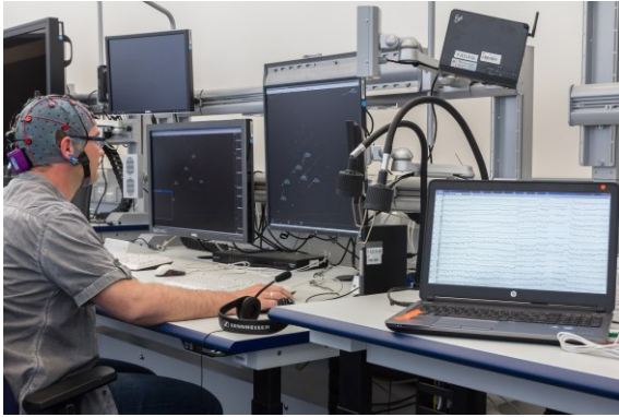
FIGURE 4. EEG Measurement in an ATC Simulation
